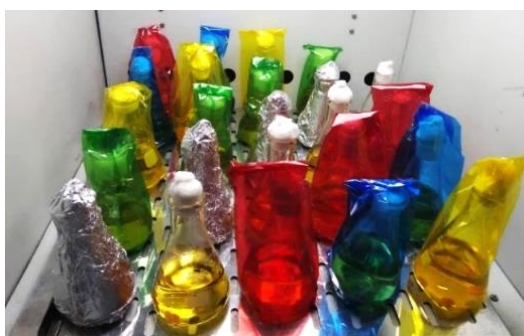
Figure 3. Experimental setup to study the effect of different light source on growth, and extracellular pigment production for Pseudofusicoccum sp.
